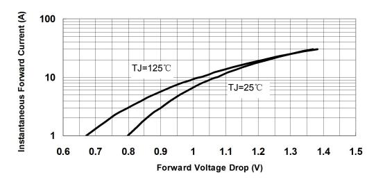
Fig.3-Typical Instantaneous Forward Voltage Characteristics
